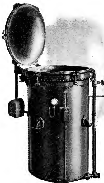
FIG. 76.—A “process kettle” (steam-pressure sterilizer) used in canning Diameter, 40 inches; height, 72 inches.
